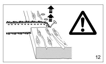
This reaction can occur in a fraction of a second and under some circumstances, cause the guide bar and chain to strike the operator with enough force to cause severe or fatal injury. It may also occur during limbing. It also occurs when the nose of the guide bar is pinched unexpectedly, unintentionally contacts solid material in the wood (fig.12) or is incorrectly used to begin a plunge or boring cut.
